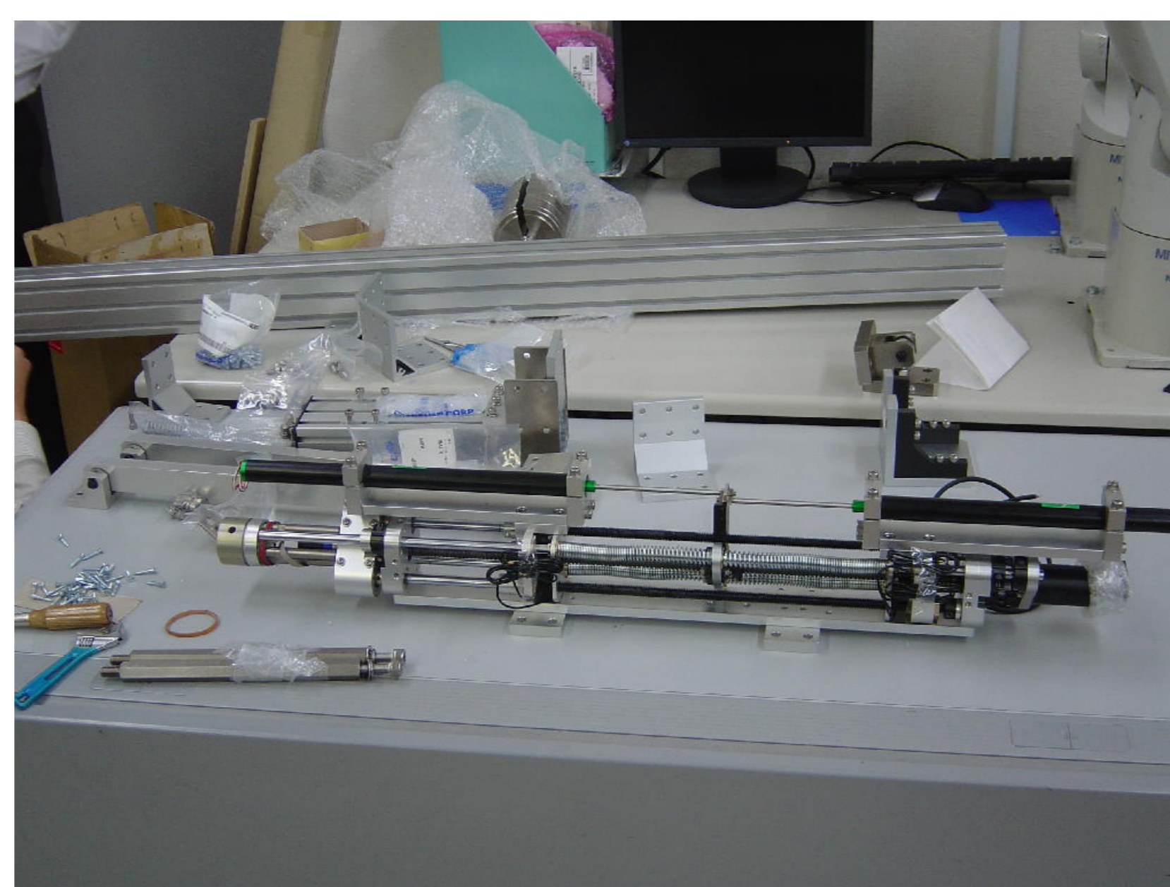
Figure 7: The VSSEA on a table. Extra sensors have been fitted to the VSSEA for testing.
